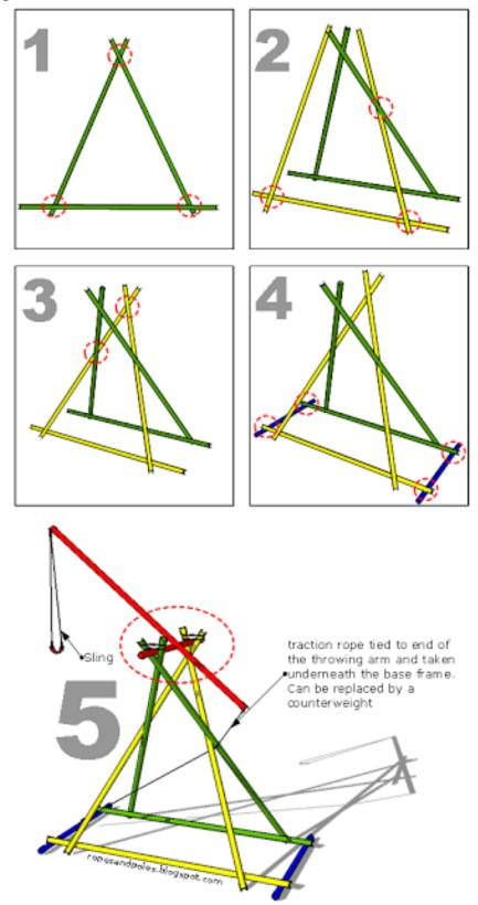
Replace traction rope with a counterweight
