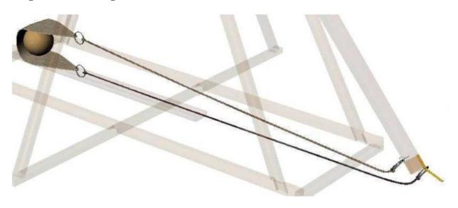
Firing Pin/Trigger Mechanism for Trebuchet
